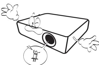
9. Never replace the light source assembly or any electronic components unless the projector is unplugged.
