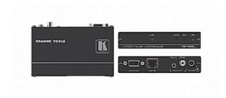
The TP-122xl is a high-performance twisted pair receiver for computer graphics video and unbalanced stereo audio signals. It converts the twisted pair input signal to WUXGA video, unbalanced stereo and S/PDIF audio signals.
