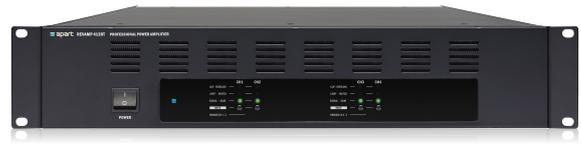
REVAMP4120T is a professional 4-channel digital power amplifier with 4 x 120 watts output power @ 100 volt (or @ 4 ohms), but the unit is also bridgeable to 2 x 240 watts @ 100 volt (or @ 4 ohms). The unit incorporates a high efficient SMPS power supply, outputs with efficient Class D output topology and output transformers.
