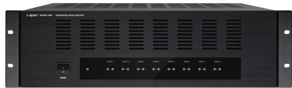
REVAMP1680 is a professional 16-channel digital power amplifier with 16 x 80 watts output power @ 4 ohms, but the unit is also bridgeable to 8 x 160 watts @ 8 ohms. This 3 rack units high amplifier with very high channel separation also has a dual analog power supply with toroidal power transformers. The standby power consumption is very low, less than 0.5 watts!
