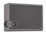
The SM6V is a functional on-wall cabinet speaker. It has a 5" paper woofer and is equipped with 100 volt power transformer with power taps on 1.5 - 3 - 6 watts.
