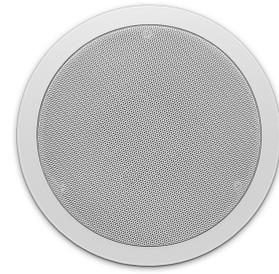
Apart CM6T is a two-way low impedance or 100 volt loudspeaker suitable for the distribution of microphone calls and background music. In 16 ohms use, you can connect up to 4 loudspeakers in parallel on each channel of a standard 4 ohms amplifier.
