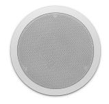
Apart CM6T is a two-way low impedance or 100 volt loudspeaker suitable for the distribution of microphone calls and background music. In 16 ohms use, you can connect up to 4 loudspeakers in parallel on each channel of a standard 4 ohms amplifier.
