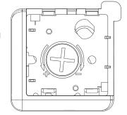
If the screen locks at the bottom and will not retract, turn adjustment knob one quarter turn counterclockwise.
