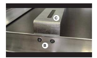
After that, mount the two iron brackets for the threaded rods using the proper holes that you find on the aluminium profile. (you will find the threaded rods inside the packaging of projector lift SI-100 or SI-200)
