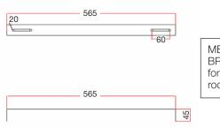
MEASURES BRACKETS for the threaded rods (in mm.)
