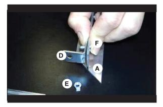
Mount the frame, fixing the four aluminium profiles by the four angle bars with bolts and nuts supplied (the nuts should be facing the internal part of the frame)
