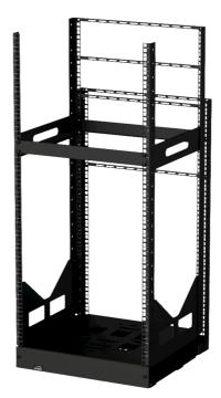
The rack shall be a 19" slide-out rack type suitable for flush mount installation use which complies to ANSI/EIA RS-310D, DIN41491 and IEC60297 standards with 24 usable rackspaces. It shall have the following dimensions: height 1145 mm, width 503 mm and depth 489 mm with a weight of kg.
