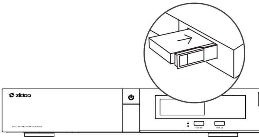
**Note:** Do not load or change the hard disk while the power is on to avoid damage of the device or hard drive data. If it is a brand-new hard disk, please format it before loading it to the device. This device supports hard disk of the following formats: EXT3, EXT4, NTFS, FAT32, EXFAT.
