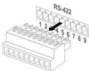
2. Peel off a section of copper wire (AWG Nos. 28 to 18) and insert it into the connector hole; then use flat screwdriver to tighten it into place.
