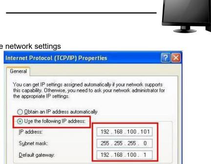
2. To connect directly through network cable, the IP address of the computer should be changed so that it is on the same network segment as the camera e.g.: The factory-preset default IP address of CV630-IP is 192.168.100.100. The computer IP address must be set with the same network segment, such as 192.168.100.101, so that the computer can be connected correctly with the camera
