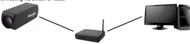
2. If the camera is connected to the computer directly, the computer IP address must be modified to have the same network segment as the camera For example, the factory-preset default IP address of CV355-30X-IP is 192.168.100.100. The computer IP address must be set with the same subnet, such as 192.168.100.101, so that the computer can be connected correctly with the camera
