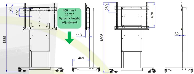
Dimensions of the Mobile Stand Mix® 481A71001 with BalanceBox®400 height adjustable mount and with VESA interface bracket 481A70 (both not included)
