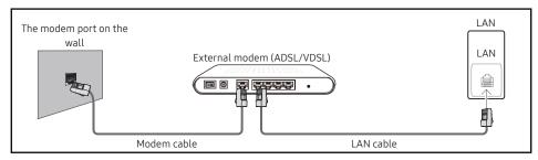
You can attach your product to your LAN by connecting the LAN port on the back of your product to an IP sharer which is connected to an external modem. Use LAN cable for the connection. See the diagram below.
