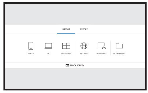
BLOCK SCREEN: You can hide the Flip screen for a while with BLOCK SCREEN. To return to the previous screen, press the Power button.
