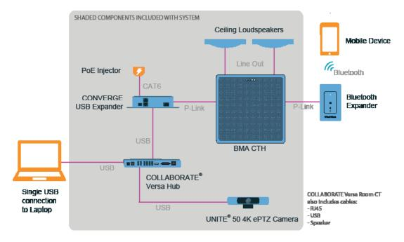
Versa Room CT using room PC and display, with optional ClearOne Wall-Mount Bluetooth Expander
