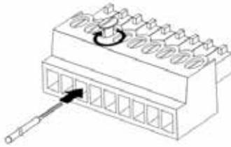
3. Insert the wired RS-422 connector back to the camera. Now the connection is completed
