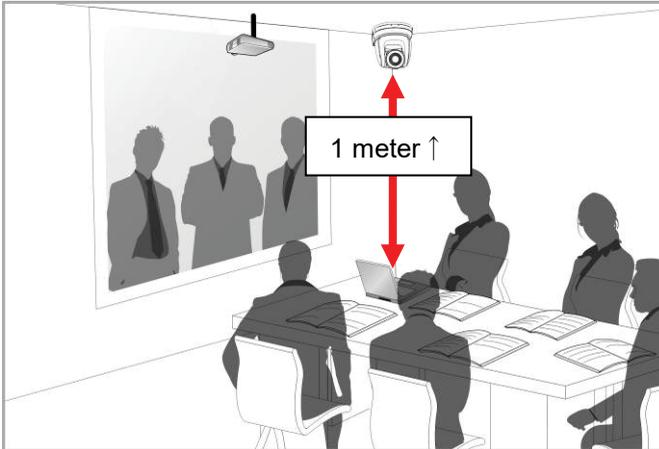
3. The machine (including metal plates) is weighed at about 2.5 kg. If it is to be installed on the ceiling, please use the hanger that has obtained UL security approval to prevent the machine from falling down.
