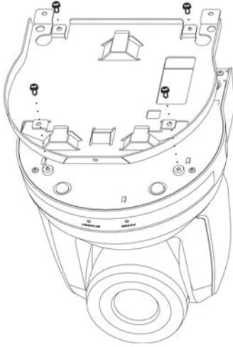
3. Lock the metal plate B on ceiling mounted hanger
