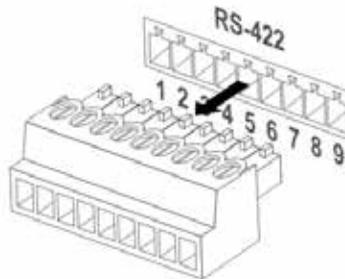
2. Peel off a section of copper wire (AWG Nos. 28 to 18) and insert it into the connector hole; then use a flat head screw driver to fix it
