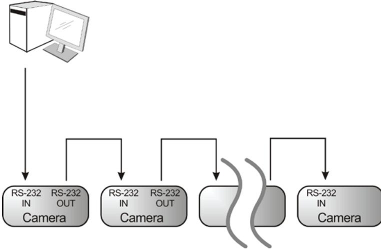
\* **With RS-232 in/out, at most 7 CVs can be connected.**
