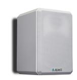
Apart VINCI Series has been expanded with a new VINCI4-16 bass reflex cabinet loudspeaker. VINCI4-16 has an impedance of 16 ohms, what allows the connection of up to 4 VINCI4-16 loudspeakers in parallel on a single amplifier channel, capable of handling a 4 ohm load.
