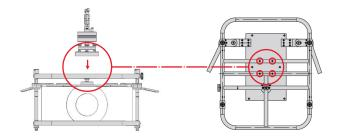
Place the truss mount on the rear side of the frame. Make sure that the 4 screws enter the 4 holes in the frame. Tighten the screws to secure the truss mount on the frame.
