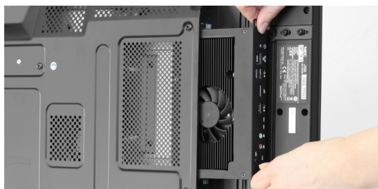
OPS Slot-in PC Installation
