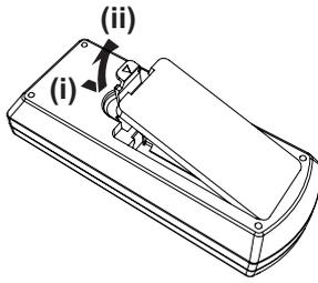
2. Remove the batteries.
