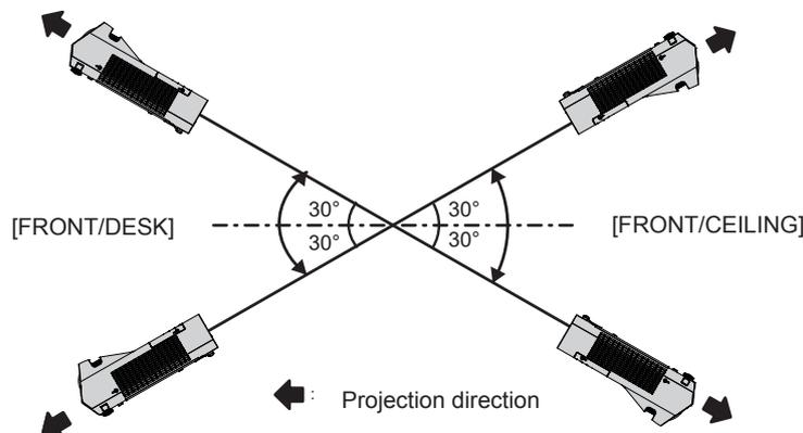
In the case of [AUTO], it will be detected as [FRONT/DESK] even when the projector tilts over  $\pm 30^\circ$  with the top side upward or over  $\pm 30^\circ$  with the top side downward. To use the projector that tilts over  $\pm 30^\circ$  with the top side downward, set the [PROJECTOR SETUP] menu → [PROJECTION METHOD] to [FRONT/CEILING] or [REAR/CEILING] instead of [AUTO].
