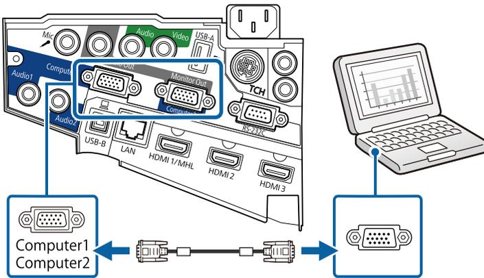
**3** Tighten the screws on the VGA connector.
