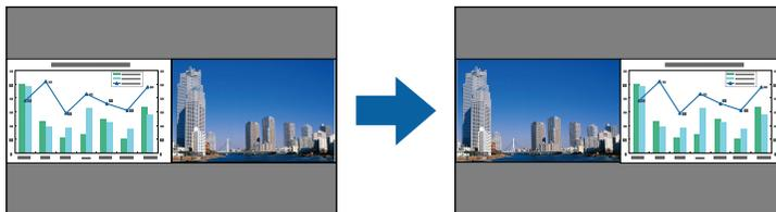
**5** To enlarge one image while reducing the other image, select **Screen Size**, press [Enter], select a size, and press [Enter]. To exit the menu, press [Menu].
