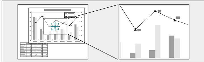
The enlarged image is projected and the enlargement ratio is displayed on the screen.
