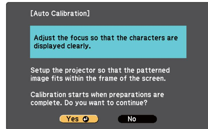
**4** Adjust the focus, if necessary, by opening the air filter cover on the side of the projector and sliding the focus lever.
