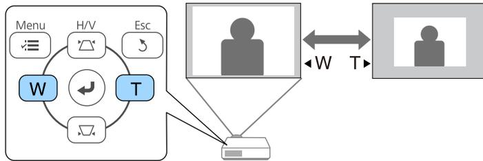
You can use the Image Shift feature to adjust the image position without moving the projector.
