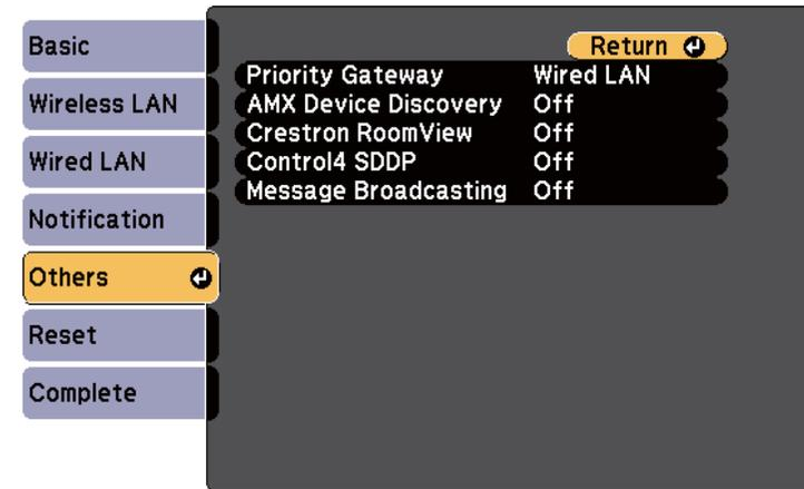
**5** Set the **Crestron RoomView** setting to **On** to allow the projector to be detected.
