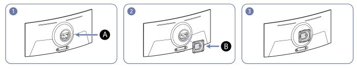
A Attach the BRACKET WALL here
