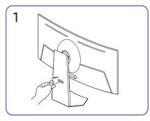
Pass cables through the hole on the stand.
