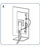
Put both cables in the cable holder on the stand (HOLDER-STAND CABLE) to organise the cables, as shown in the figure.
