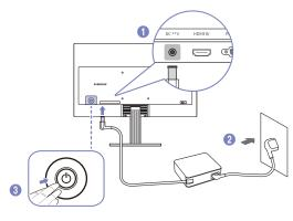
1 Connect the power cord to the AC/DC adapter. Then, connect the AC/DC adapter to the DC **\*\*V** port on the back of the product.
