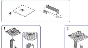
Put the stand base onto the stand neck as the direction shown in the figure. Check that the stand neck is firmly connected.
