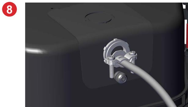
9. Secure a safety cable to the seismic safety tab. Make the cable as short as possible. Attach the cable to a secondary structural point directly above the seismic safety tab to minimize impact force and swing in the event of a ceiling failure.
