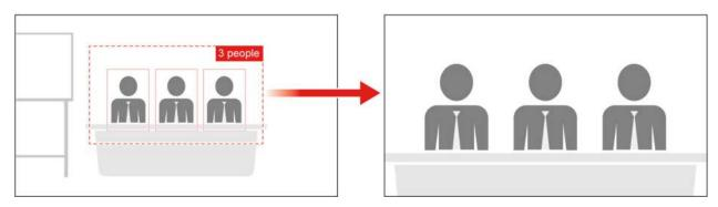
• **Speaker tracking and whiteboard recognition**: Auto track the speaker and count the whiteboard nearby as a person. Then auto frame and zoom in the speaker and the whiteboard to a suitable size. The camera will use Picture-in-Picture mode to replace the original video image in the sub image. This function makes the conference more focus on the speaker and the content of whiteboard.
