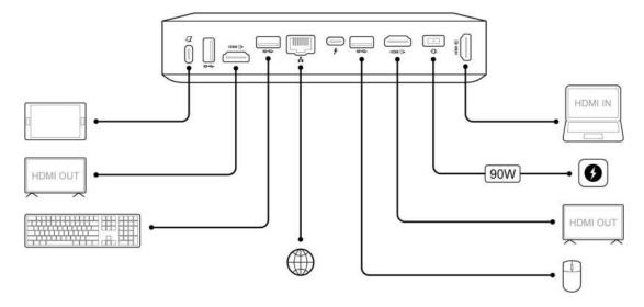
**Note:** Ensure that you connect your computer to the HDMI-in connector (**HDMI** $\rightarrow$ ) and connect the external displays to the HDMI-out connectors (**HDMI** $\rightarrow$ ).
