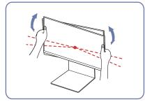
• Hold the bezel at both side edges and adjust the monitor angle until the screen becomes level. (Be careful not to directly hold the LCD display.)
