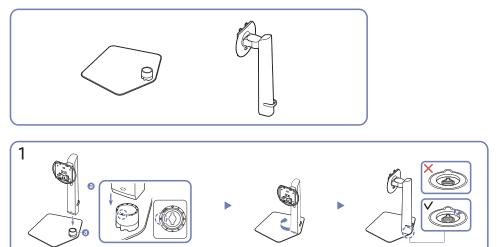
Check the direction of the arrow on the stand base. Align the direction of the arrow on the stand base with the front direction of the stand neck, and then insert the stand neck from top to bottom. Turn the stand neck clockwise to fasten it to the base. Lift the stand slightly and check that the PUSH button on the bottom of the base protrudes.
