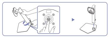
Lift the assembled stand slightly and press the PUSH button on the bottom of the base. While holding down the PUSH button, turn the stand neck anticlockwise to remove it.
