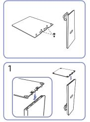
Put the stand base onto the stand neck as the direction shown in the figure. Check that the stand neck is firmly connected.
