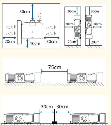
If there is not enough space around the projector and the internal temperature of the projector increases, the brightness of the light source may decrease.
