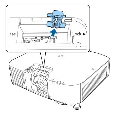
4. Pinch the lock lever and move it to the **Release** position.
