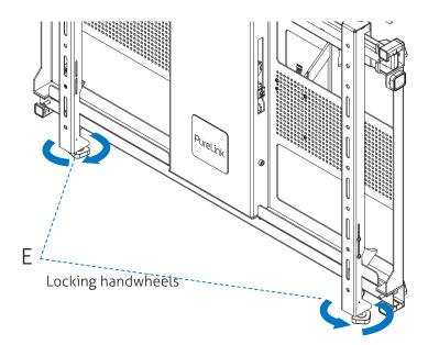
\*Note: Locking handwheels must be loosened before any adjustments can be made. Once all adjustments are done, the locking handwheels can be tightened.
