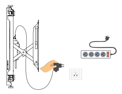
Note: Once the screens are installed, aligned and closed, to prevent accidental movement of the Mount or electrical interference/damage, ensure that Mount-dedicated power strips or power supply is turned off/unplugged, until next service appointment.
