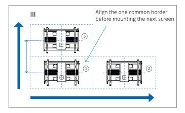
Height of screen determines center to center distance for next vertical mount location.
