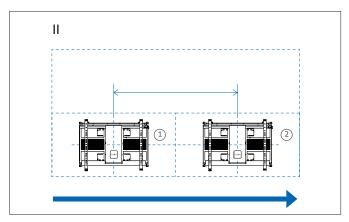
Width of screen determines center to center distance for next horizontal mount location.
