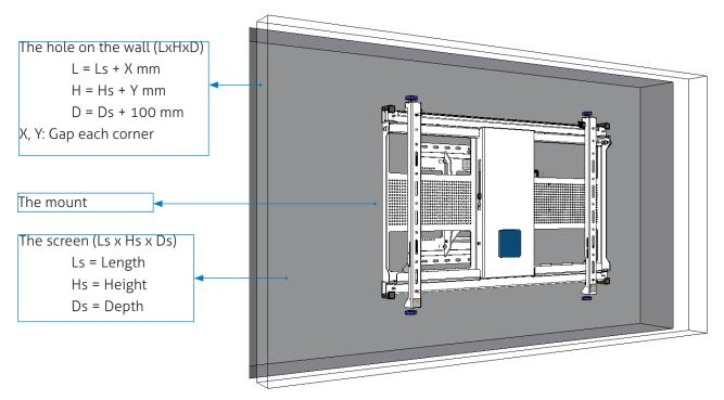
The dimension of rectangular holes on the wall need to be created based on the screen's dimensions. Note: Some screen manufacturers do not put the VESA holes at the center of the screen backside. Therefore, you should locate the position of back wall plate and mark the drill holes with the following instruction.
