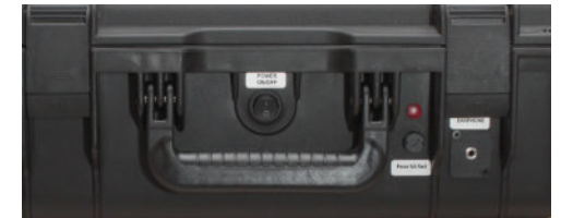
(Image 21) LED & fuse on the frontside of an ATEM Extreme Case
