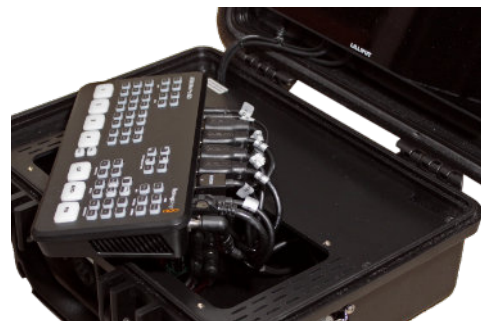
(Image 12) Plug the cable into the ATEM
