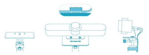
Fasten Tripod Mount to Tripod
