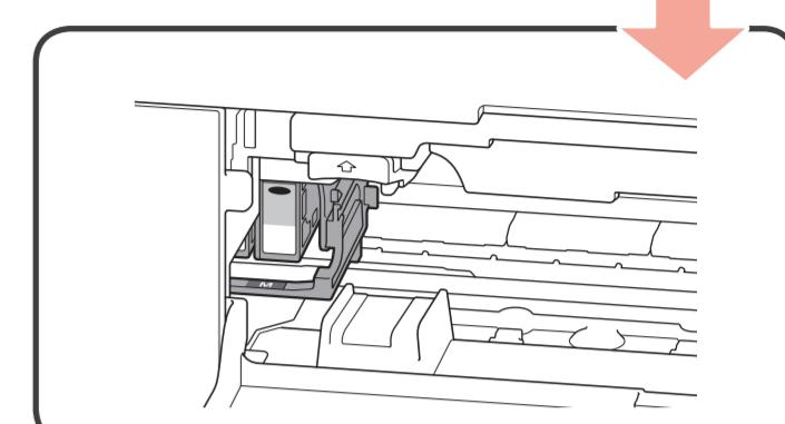
An installed ink tank cannot be removed until the message to replace it is displayed.
