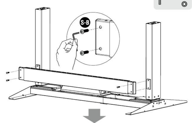
Reinsert the previously removed screws and tighten them all.
