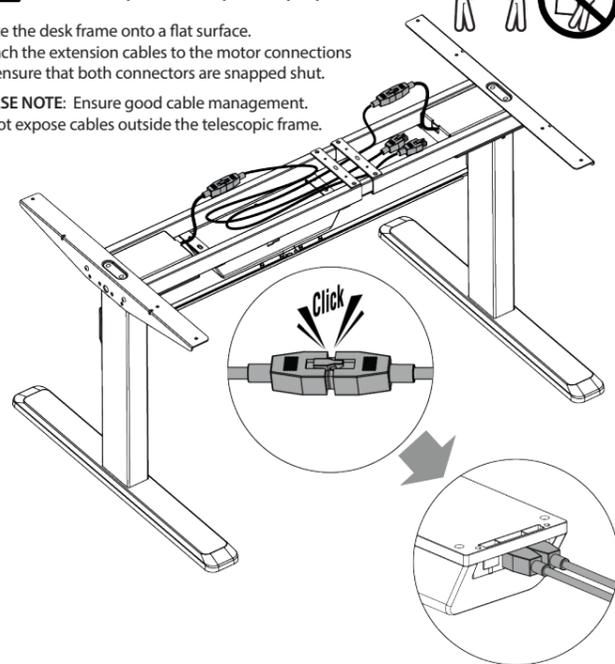
Connect the extension cables to the motor connection ensuring they click together securely.
