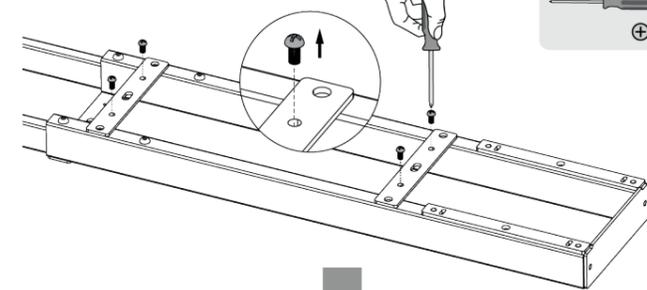
Attach the control unit to the frame using the screws previously removed. Tighten all screws.
