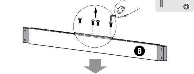
Adjust the cross bar so that the mounting holes of the lifting columns are aligned and tighten the four screws.
